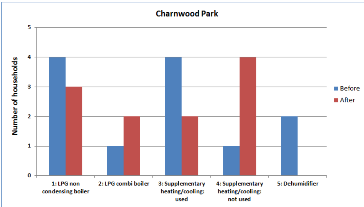
Figure 2.11 Changes in boiler type, useage of supplementary heating/cooling and dehumidifier, before/after
