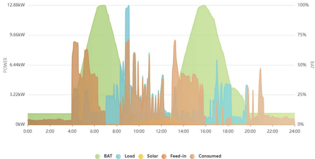
Figure 2.13 Power Diagram from the Alpha ESS battery portal for Household B-03 on Sunday 29 Dec 2024 with the EDF heat pump tariff
