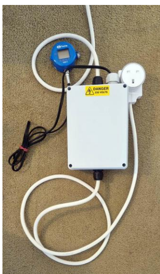
Figure 1.10 Monitoring lead for Tiny Tag View 2 data logger
