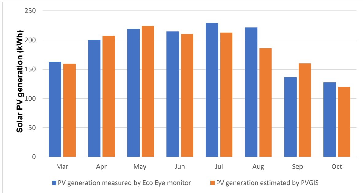
Figure 4.34 Monthly PV generation for household E-02 measured by the Eco Eye monitor and estimated using PVGIS
