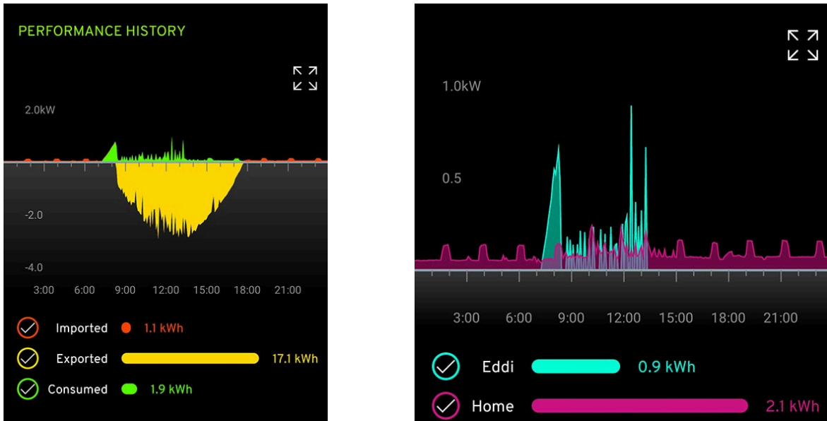
Figure 4.14 Images from the myenergi app on 18 Mar 22, a sunny day with the resident not at home
