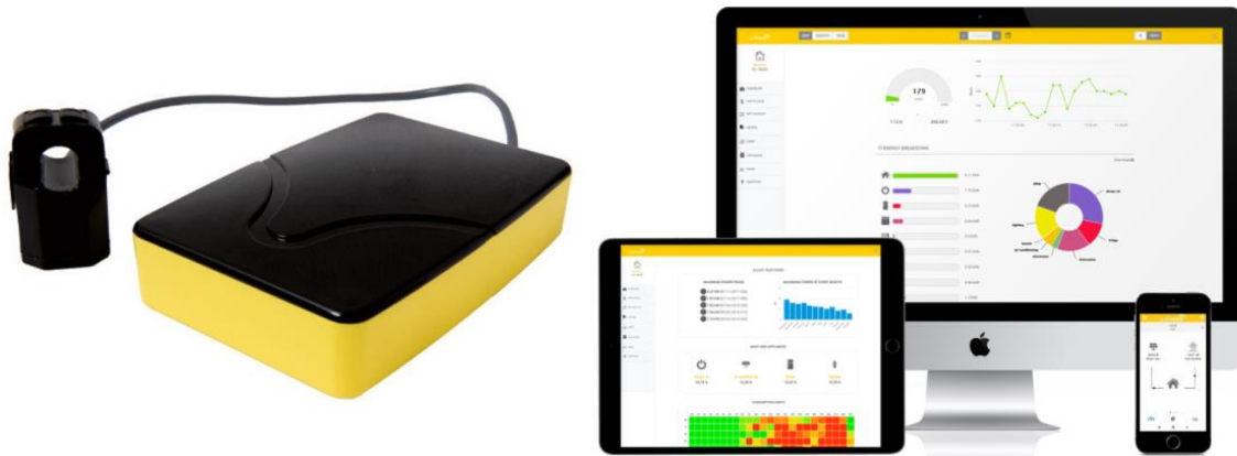
Figure 3.19 Wibeec Box logger and CT clamp with images from the Wibeec Home app and portal
