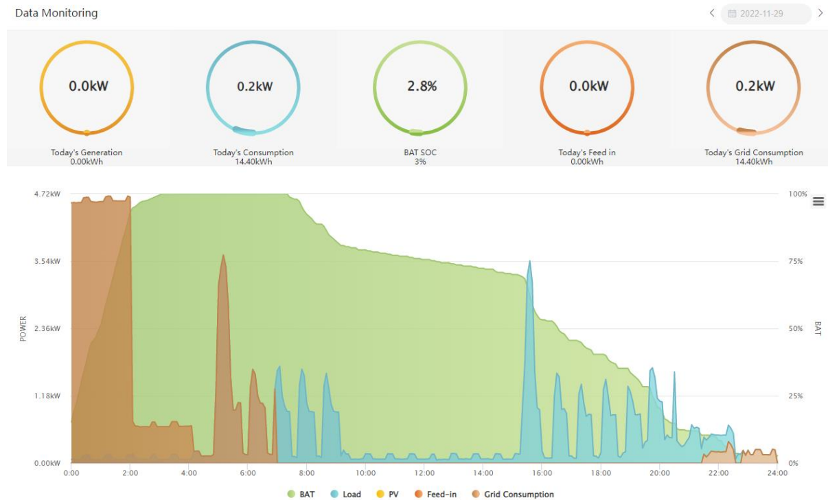
Figure 3.13 Power diagram from the Alpha ESS battery monitoring portal
