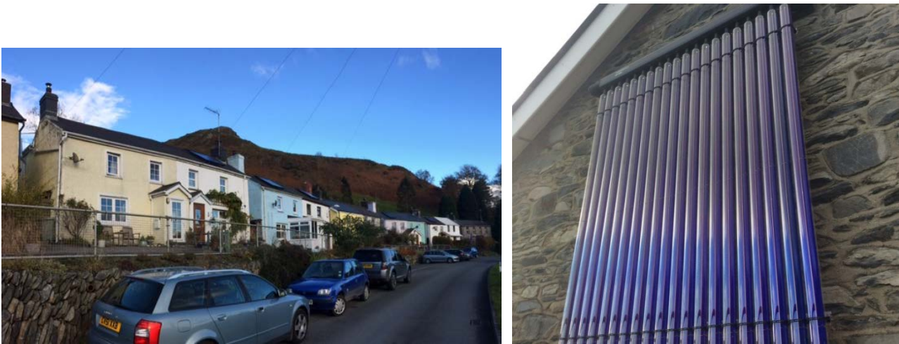
Figure 1.3(a) left, solar thermal panels on south facing roofs at New Row and (b) right, wall-mounted solar thermal panel
