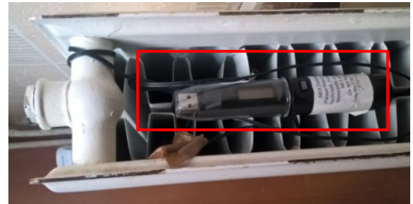
Figure 2.3 Lascar EL-USB-2 temperature and humidity logger (left) and thermal probe (right)
