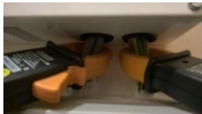
Figure 4.7 showing an example of clamps around multiple cables
