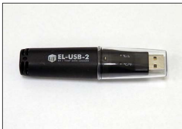
Figure 3.1 Lascar EL-USB-2 temperature and humidity logger
