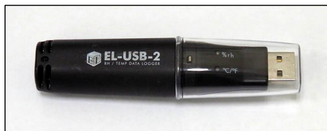
Figure 3.6 Lascar EL-USB-2 temperature and humidity logger
