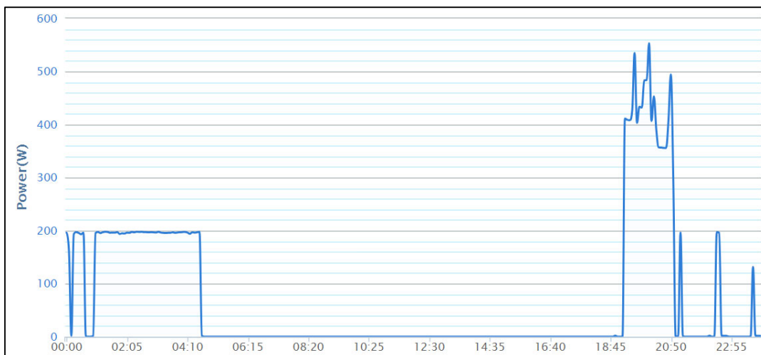
Figure 3.82 Plot of battery discharge against time on 27 Apr 2018 for household T-27
